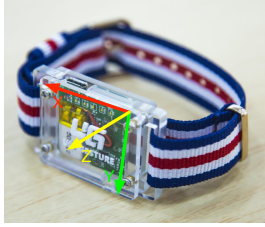
(b) Coordinate System of a UG wristband
