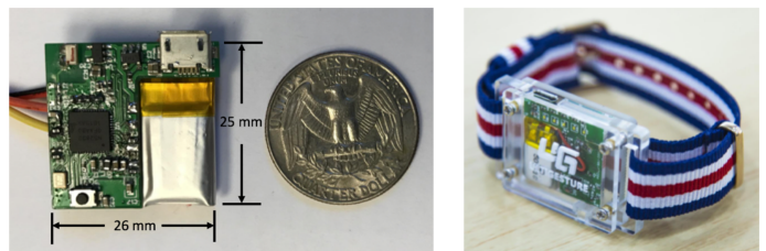
Fig. 3: UG Sensor band: A combination of accelerometer, gyroscope, magnetometer
